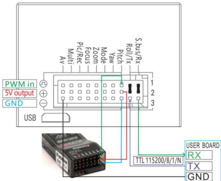
S.bus/Rx: connect to Rx2 for track function.
