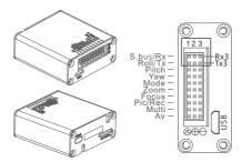
To use the serial port function, please use the jumper cap to connect RX1 and RX2, TX1 and TX2.
