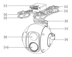
[1]Control box [6]YAW axis motor
