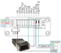
S.bus/Rx:connect to Rx2 for track function.
