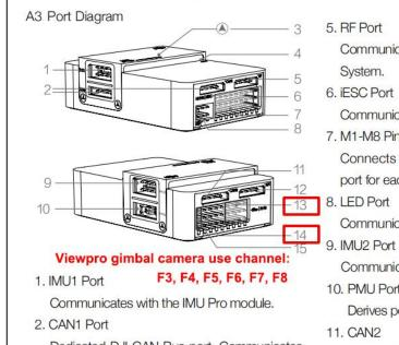
Dedicated DJI CAN-Bus port. Communicates with the A3 GPS-Compass Pro or other DJI devices (e.g. Real Time Kinematic (RTK) GPS
