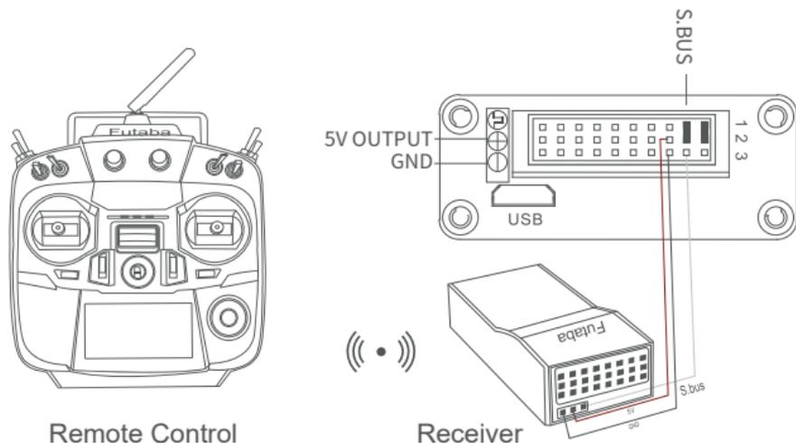
Wiring Diagram Standard Version
