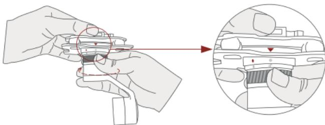
4. To unlock the Viewport, you need to press on unlock button and rotate the gimbal camera clockwise till the white dot align to the red triangle. Then pull the gimbal out from the Viewport.
