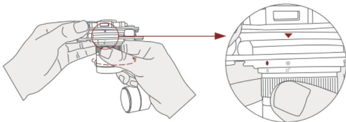
2. Align the white dot (unlock icon) to the red triangle (below unlock button), push the gimbal into the Viewport completely and then rotate the gimbal camera anticlockwise.
