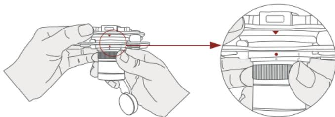
3. When you hear "click" sound (when red dot is aligned to the red triangle) means the gimbal camera and Viewport has been locked.
