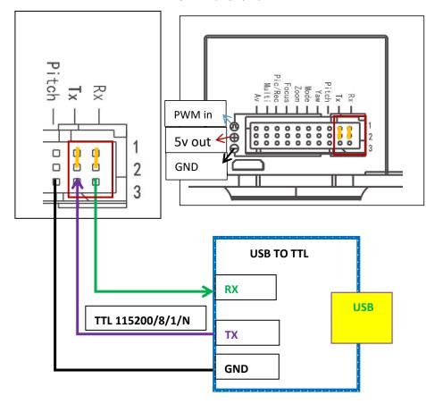
RX1/ RX2 and TX1 / TX2 must be connected with jumper caps before connecting UART/FTDI devices.
