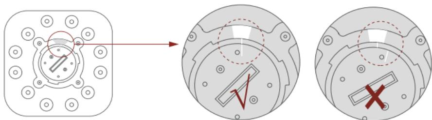
1. Make sure the two white stripes indicated in above picture are aligned with each other. (If the stripes are not aligned to each other, please pinch the connector part and turn it to left manually)
