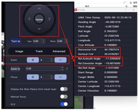
6. Connect gimbal serial port to FC, make sure gimbal can get GPS from FC, the time data will also be changing. According the document 《Settings for the open-source Viewlink Gimbal Docking.pdf 》.
