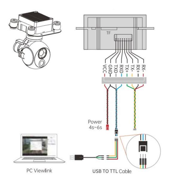
Then power on the Gimbal Camera , open the software interface, click "Connect" and select the corresponding serial port COMX on the computer equipment manager, the default baud rate is: 115200, and then click "Connect", the control bar corresponding to the Viewpro" Gimbal Camera model appears on the right side of the ViewLink interface, at this time the Gimbal Camera can control the gimbal and camera function.
